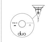
input signal wired directly to base of duo
